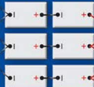
Configuration 3 Double Voltage Increase Capacity by 3X's
